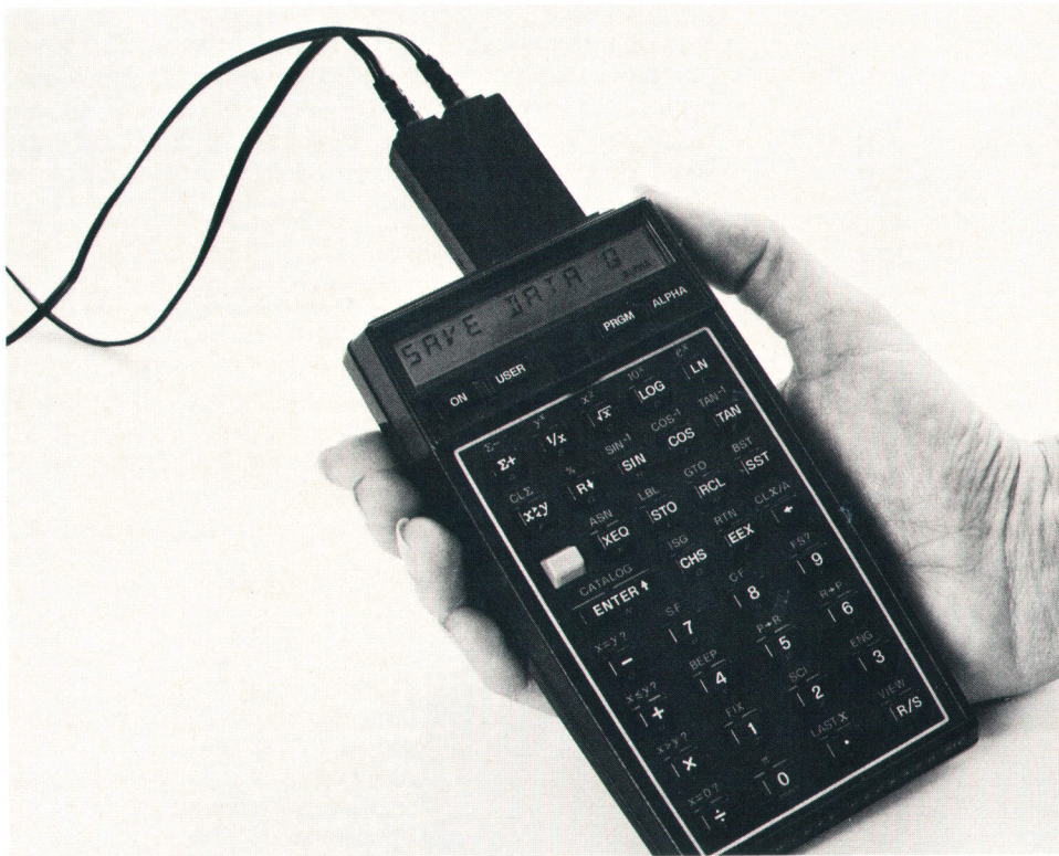
Fig. 5. When a user plugs the HP 82160A HP-IL Module into one of the four I/O ports in the HP-41CV Programmable Calculator, the calculator becomes a portable system controller, able to interface with a variety of peripherals. Through the HP-IL, the HP-41CV can control a graphics plotter (see last month's issue, page 16), display data on a video monitor, transmit data over telephone lines to a larger Series 80 Computer, and collect measurements in the field.
